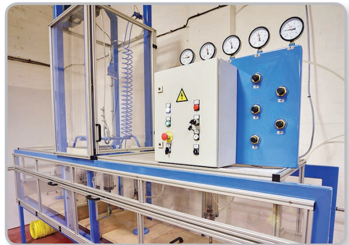
In-house trench test ensures EN12613 compliance.
